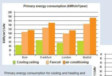
Primary energy consumption for cooling and heating and ventilation as a result a EnergyPlus simulation of a typical office building (511m²). The building is satisfy national energy standards. For heating it was used gas assist technology. For cooling it was used air cooling technology. But in case of cooling and heating ceiling ther was adding of groundwater allowed.
